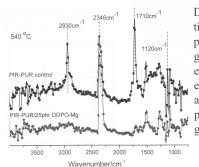
DOPO–Mg changed the thermal degradation process of the PIR–PUR foam and prevented a kind of highly toxic flammable gas from being generated. DOPO–Mg can effectively produce spherical material covering the surface of the char to hinder flame and energy transmission in the condensed phase. The FTIR spectra of the pyrolytic gas products at 540 °C.
