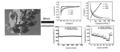
A porous N-doped carbon has been fabricated through a convenient, economical, and scalable route without the assistance of any activation or template technique. The biomass derived porous carbon delivers high reversible capacity (505 mAh•g<sup>-1</sup> at 0.1 C), excellent rate capability (190 mAh•g<sup>-1</sup> at 10 C), suggesting that the as-obtained carbon can be a promising anode material for lithium ion batteries (LIBs).
