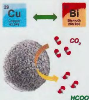
Bimetallic Cu-Bi  $\text{CO}_2$ RR electrocatalysts were prepared via the cathodic conversion of hierarchical  $\text{CuBi}_2\text{O}_4$  microspheres. They enabled the high-performance electrocatalytic reduction of  $\text{CO}_2$  to formate with large current density, excellent selectivity, and sufficient durability.
