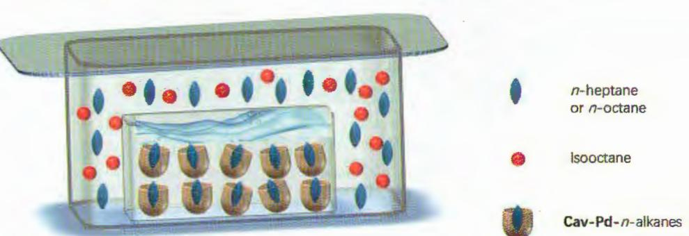
Metallo cavitand aqueous solution (Cav-Pd) selectively adsorb *n*-alkanes from their mixed vapor with isooctane.
