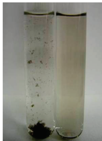
FIGURE 4. Photograph of 10 mg/L SWNT-COOH in water at pH 3: A sample irradiated with lamp light ( \lambda = 350 \pm 50 \text{ nm} ) for 6 h is on the left and the dark control sample is on the right.
