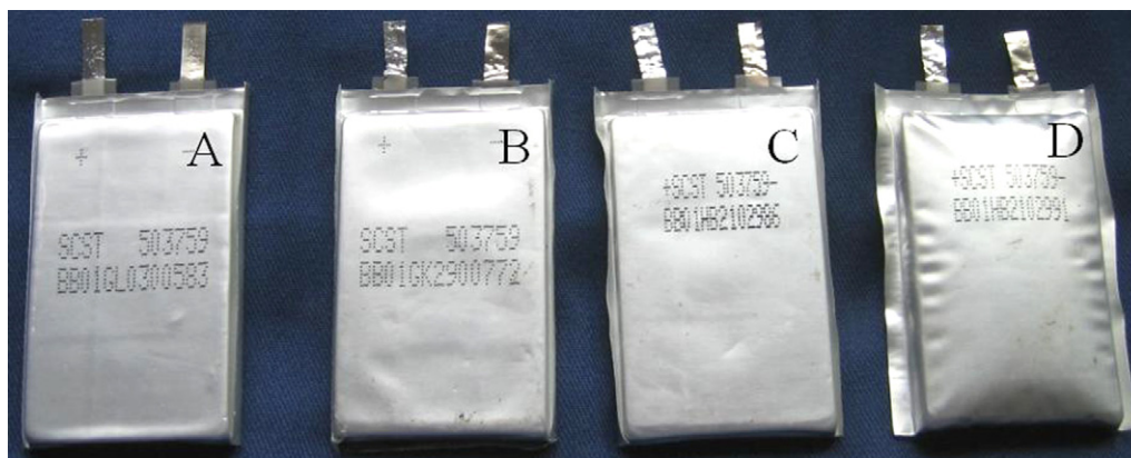
Fig. 1. Photographs of Li-ion cells after storage at 55 °C for 100 days. (a) Fresh cell; (b, c and d) cells stored in 0, 50 and 100% SoC, respectively.
