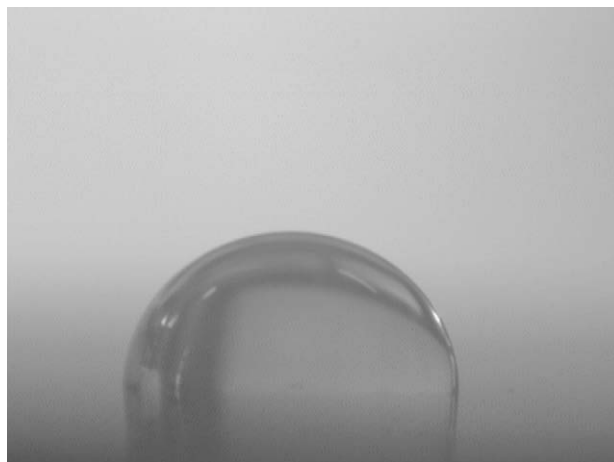
Fig. 7 – Contact angle of the coated bipolar plate with water.
