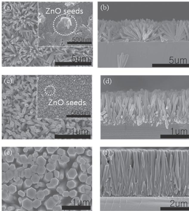
**Fig. 2.** SEM images of surface and cross-sectional morphologies of ZnO NRs; (a, b) flower shape, (c, d) askance shape, and (e, f) vertical shape. The inset shows SEM images of morphologies of ZnO seed for (a) flower-shaped NRs, (c) vertical and askance-shaped NRs, respectively.
