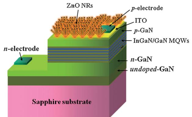
Fig. 1. Schematic view of LED device structure with various shapes of ZnO NRs.
