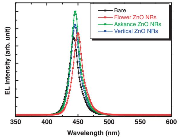
**Fig. 4.** EL spectra of LEDs with various shapes of ZnO NRs measured on top of LEDs.
