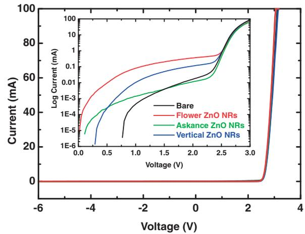
**Fig. 3.**  $I$ – $V$  characteristics of LEDs with various shapes of ZnO NRs. The inset shows  $I$ – $V$  characteristics on a log scale.
