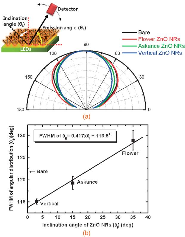
**Fig. 5.** (a) Angular dependence of EL emission intensity for LEDs with various shapes of ZnO NRs. The inset shows a schematic view of sample geometry for the measurement. (b) Plot of FWHM of the angular-dependent EL intensity, as a function of the inclination angle of ZnO NRs.
