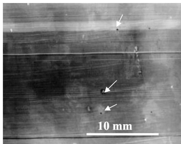
Fig. 3. Surface of Fe-32.3Mn-8.54Al-1.31Si-0.54C alloy after immersion test in alcohol fuel. Arrays indicate corrosion pits.
