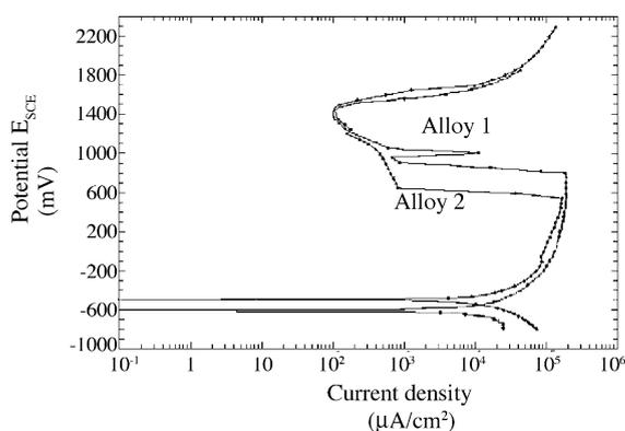
Fig. 7. Polarization curves for Fe–Mn–Al–Si–C alloys in 1N H<sub>2</sub>SO<sub>4</sub> solution.
