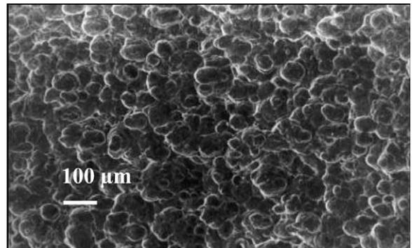
Fig. 6. Surface of Fe–32.3Mn–8.54Al–1.31Si–0.54C alloy after immersion test in lactic acid. The white area was enriched in aluminum in relation to the alloy surface.
