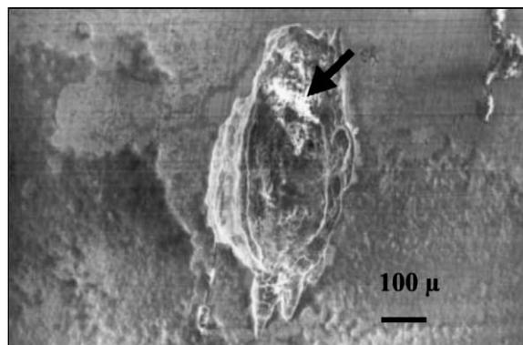
Fig. 4. Surface of the FMA alloy with 0.25% C. The white area presented a higher Al content than the alloy surface.
