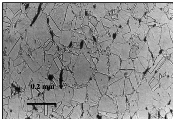
Fig. 1. Longitudinal section of the Fe–32.7Mn–6.59Al–1.26Si–0.25C (wt.%) alloy.
