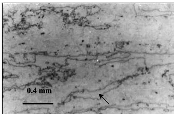
Fig. 2. Longitudinal section of the Fe-32.3Mn-8.54Al-1.31Si-0.54C (wt.%) two-phase alloy. Array indicates the ferrite phase.
