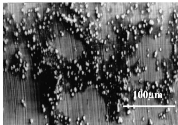
Fig. 5. Surface of Fe–32.3Mn–8.54Al–1.31Si–0.54C alloy after immersion test in boiler water.
