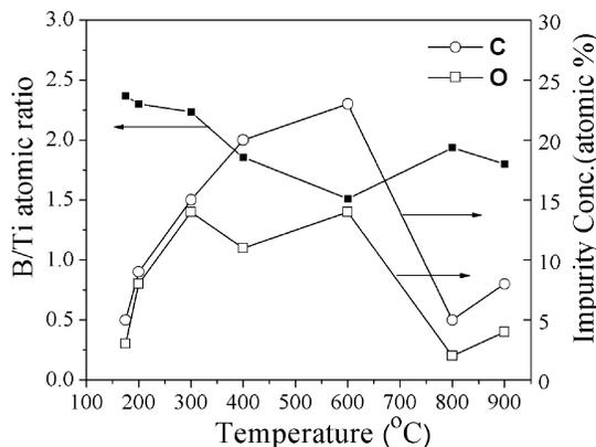
**Figure 3.** Boron to titanium atomic ratio (solid squares) and atomic concentration of carbon (open circles) and oxygen (open squares) as a function of growth temperature.
