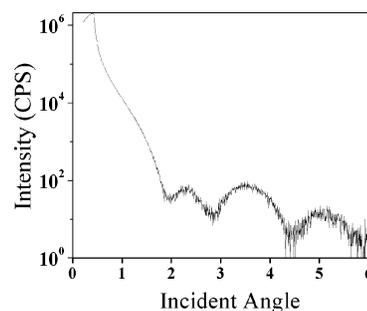
**Figure 1.** XRR measurement of a film grown at 175 °C for 1 min on SiO<sub>2</sub>. Film thickness calculated from interference fringes is 5 nm.
