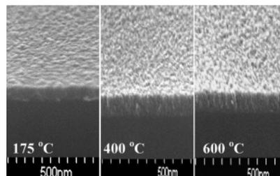
**Figure 4.** Cross-sectional SEM images of films grown at 175 °C, 400 °C, and 600 °C.
