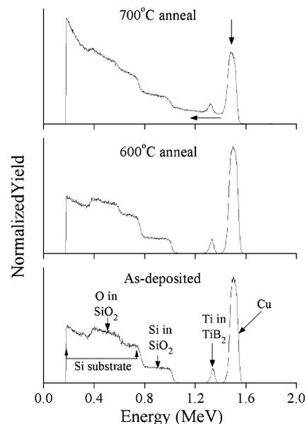
**Figure 9.** RBS profile from a diffusion test structure consisting of (40 nm) Cu/(7 nm) TiB<sub>2</sub>/350 nm SiO<sub>2</sub>/Si, as-deposited (bottom), vacuum-annealed at 600 °C for 30 min (middle), and vacuum-annealed at 700 °C for 30 min (top). The arrows in the 700 °C spectrum show the change in the shape of the copper peak due to diffusion deeper into the structure.
