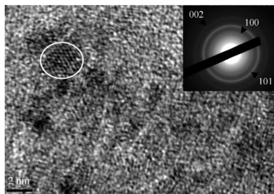
**Figure 7.** High-resolution TEM image of TiB<sub>2</sub> film grown on a Cu/SiO<sub>2</sub> grid at 175 °C; a nanocrystallite is shown encircled. Selected area electron diffraction pattern (SAED) of the same is shown in the inset with labeled TiB<sub>2</sub> lattice planes.
