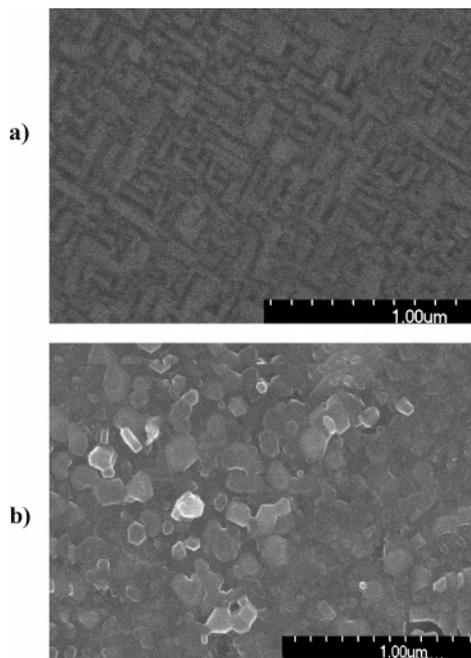
**Figure 8.** Plan view SEM images of films grown at (a) 800 °C and (b) 900 °C.
