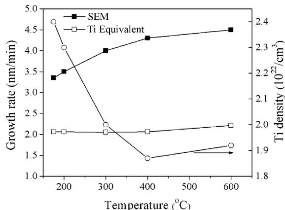
**Figure 2.** Film growth rate (solid squares), Ti-equivalent growth rate (open squares), and titanium atomic density (open circles) as a function of temperature.
