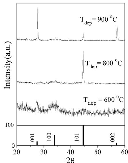
**Figure 6.** XRD profile of films grown at 600, 800, and 900 °C. The bottom of the figure shows a histogram of the ICCD X-ray powder diffraction pattern.
