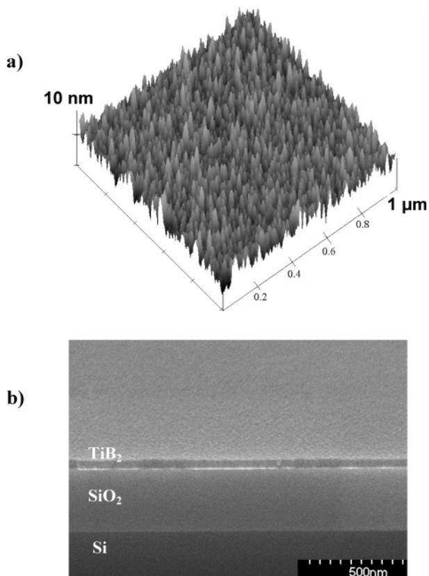
**Figure 5.** (a) AFM surface plot and (b) cross-sectional SEM images of a film grown on SiO<sub>2</sub> at 175 °C.
