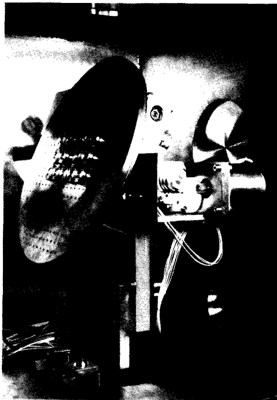
Fig. 1. The general-purpose water-cooled sample manipulator with coupon samples mounted.
