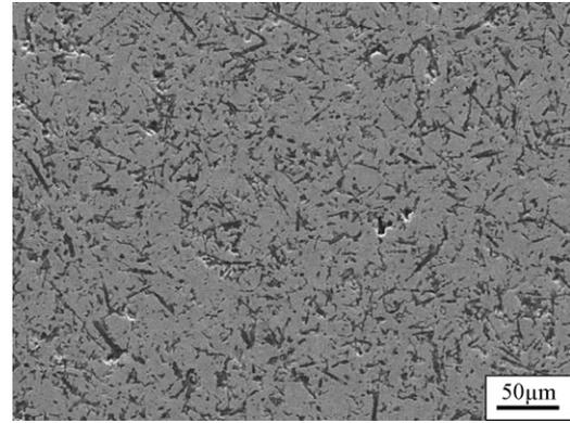
Fig. 8. SEM micrograph from a polished cross-section of the  $\text{ZrB}_2$ -SiC<sub>w</sub> hot-pressed at 1800 °C.
