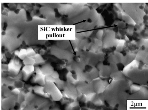
Fig. 10. SEM micrograph of the fracture surface of  $ZrB_2$ - $SiC_W$  hot-pressed at  $1800^\circ C$ .
