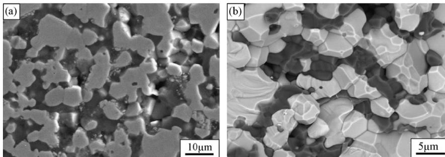
Fig. 2. SEM micrographs of the polished (a) and fracture (b) surface of  $ZrB_2$ - $SiC_W$  composites.
