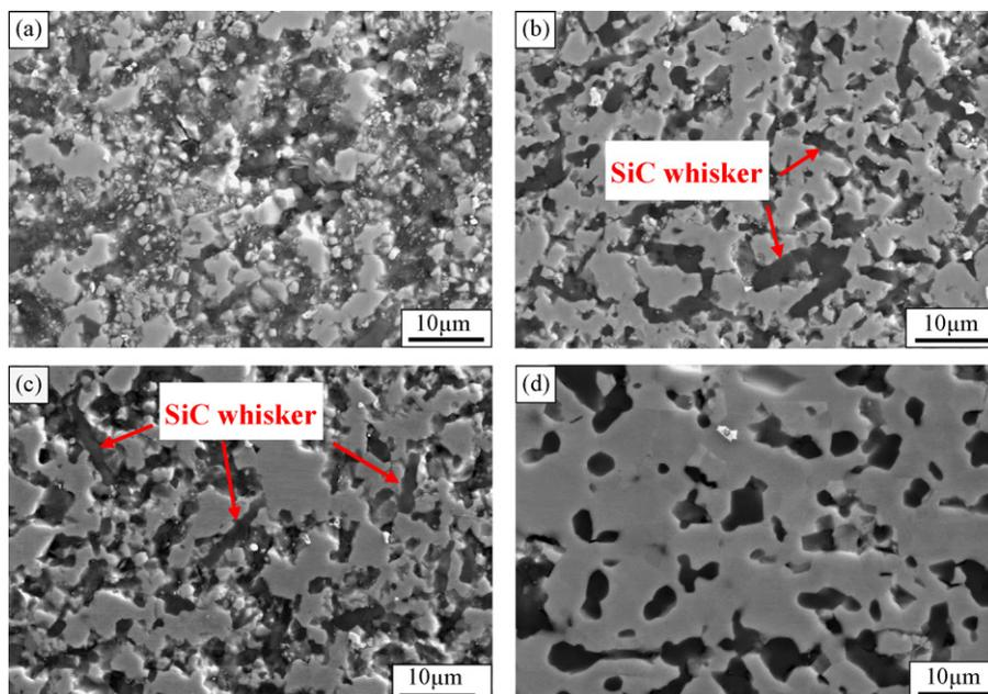
Fig. 7. SEM micrographs of  $\text{ZrB}_2$ -SiC<sub>w</sub> composite sintered at different temperatures: (a) 1750 °C; (b) 1800 °C; (c) 1850 °C; (d) 1900 °C.
