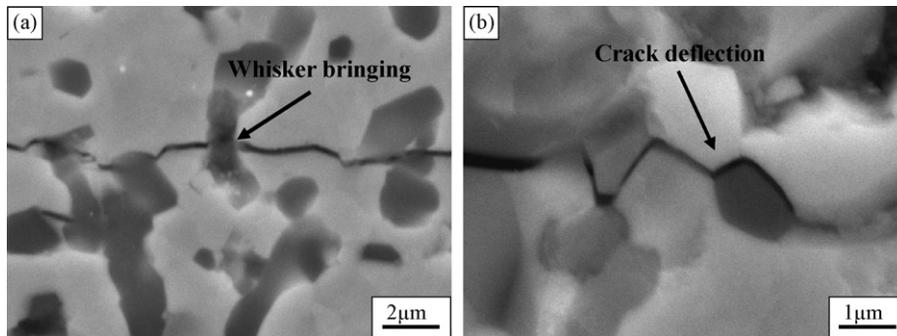
Fig. 9. SEM micrograph of the crack propagation from the Vickers indentation for the  $ZrB_2$ - $SiC_W$  hot-pressed at  $1800^\circ C$ : (a) whisker bridging and (b) crack deflection.
