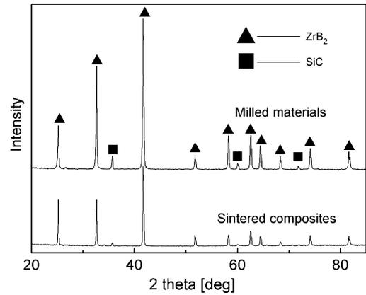
Fig. 3. XRD patterns of  $ZrB_2$ - $SiC_W$  milled materials and sintered composites.
