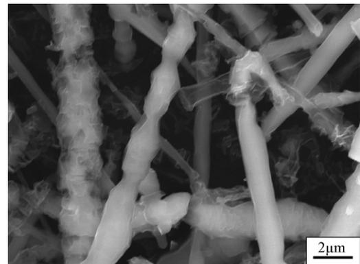
Fig. 4. SEM micrograph of the heat-treated  $SiC$  whiskers.
