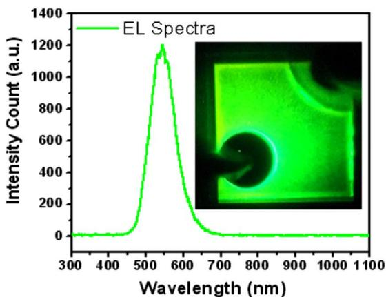
FIG. 2. (Color online) Room temperature EL spectra of the InGaN/GaN SMNG LED at a forward injection current of 10 mA. The inset image is the optical micrograph showing the green light emission across the mesa.
