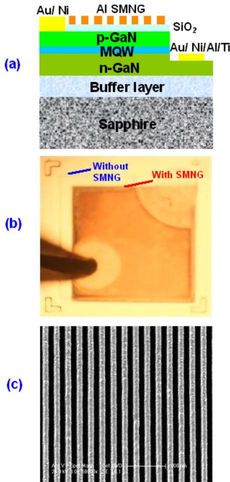
FIG. 1. (Color online) (a) Schematic diagram of the cross section of the InGaN/GaN SMNG LED. (b) Optical micrograph of fabricated SMNG LED mesa, where the SMNG patterning area appears as darker square. (c) Scanning electron microscope image of SMNG with a grating period of 150 nm.
