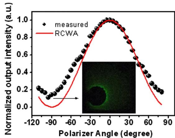
FIG. 3. (Color online) EL intensity of the InGaN/GaN SMNG LED as a function of the polarizer-rotating angle within one period range. Dots are measured with 5-degree intervals while red curve is simulated by RCWA also with 5-degree intervals but connected as a continuous curve. The inset image shows optical micrograph of the eclipselike light emission around the  $p$ -pad when polarizer angle is placed at extinction position.
