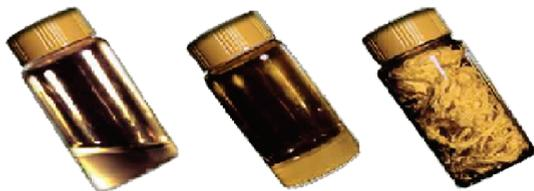
**Figure 2.** Polypropylene samples prepared by the Zr-, Hf-, and Ti-Salan catalysts (left to right).
