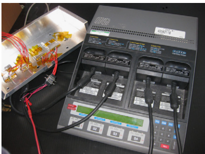
Fig. 4. Battery test setup using Cadex analyzer.
