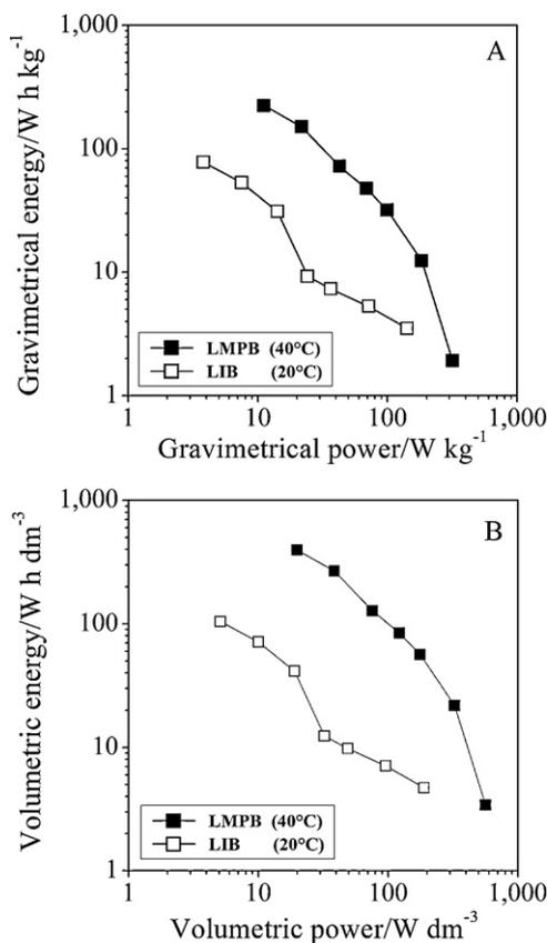
**Fig. 7.** Ragone plot in terms of gravimetric energy vs. gravimetric power (panel A) and volumetric energy vs. volumetric power (panel B) of scaled-up Li/LiFePO<sub>4</sub> (LMPB) and Li<sub>4</sub>Ti<sub>5</sub>O<sub>12</sub>/LiFePO<sub>4</sub> (LIB) battery prototypes. The energy and power data were calculated on the basis of the results obtained from cycling tests but taking into accounts on the optimization described in the text.
