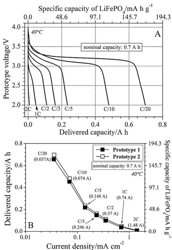
**Fig. 3.** Voltage vs. discharge capacity profiles (panel A) and discharge capacity vs. current density dependence (panel B) of scaled-up, ionic liquid-based, Li/LiFePO<sub>4</sub> LMPB prototypes. The capacity was also reported with respect to the LiFePO<sub>4</sub> active material weight for comparison purpose. The average discharge current values (and the corresponding discharge rates) are also indicated in the panels.  $T = 40^\circ\text{C}$ .
