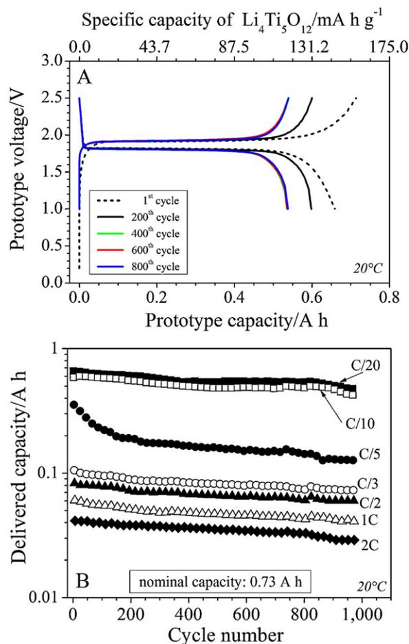
**Fig. 6.** Voltage vs. capacity profile of selected charge/discharge cycles at C/20 (panel A) and capacity vs. cycle evolution (panel B) of a scaled-up, ionic liquid-based,  $\text{Li}_4\text{Ti}_5\text{O}_{12}/\text{LiFePO}_4$  LIB prototype at different current rates.  $T = 20^\circ\text{C}$ .
