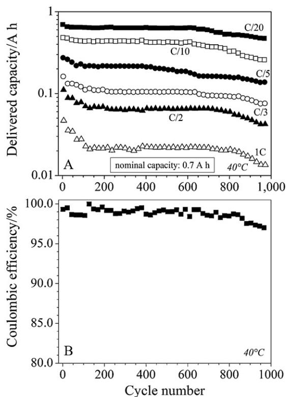
**Fig. 4.** Discharge capacity (panel A) and coulombic efficiency (panel B) evolution of a scaled-up, ionic liquid-based, Li/LiFePO<sub>4</sub> LMPB prototype at different current rates.  $T = 40^\circ\text{C}$ .
