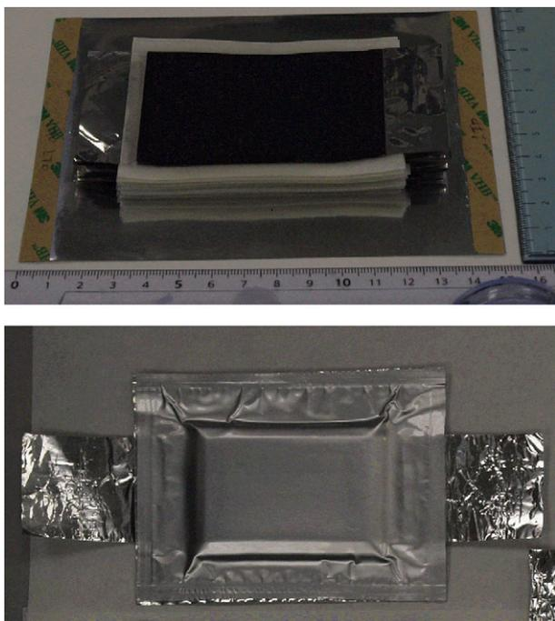
**Fig. 1.** Picture of a scaled-up, ionic liquid-based,  $\text{Li}_4\text{Ti}_5\text{O}_{12}/\text{LiFePO}_4$  LIB prototype before (upper panel) and after housing in vacuum-sealed pouch-bag (lower panel).
