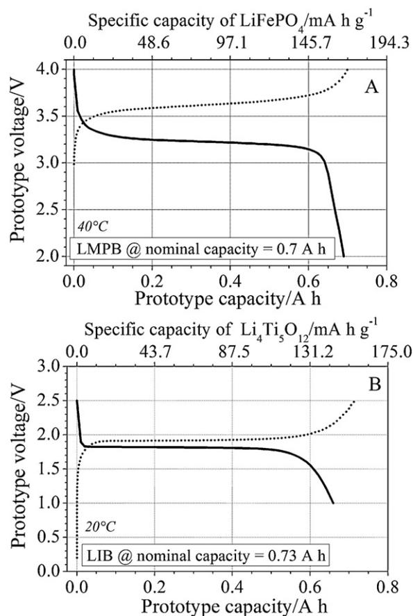
**Fig. 2.** Voltage vs. capacity profile of the 1st charge-discharge cycle for a scaled-up, ionic liquid-based,  $\text{Li}/\text{LiFePO}_4$  LMPB (panel A) and  $\text{Li}_4\text{Ti}_5\text{O}_{12}/\text{LiFePO}_4$  LIB prototype (panel B). Current rate: C/20. In the upper axis is indicated the capacity of the  $\text{LiFePO}_4$  (panel A) and of the  $\text{Li}_4\text{Ti}_5\text{O}_{12}$  electrode (panel B) for the LMPB for the LIB prototype, respectively.
