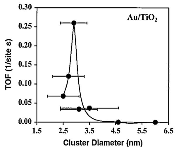
**Fig. 7.** CO oxidation turnover frequencies (TOF) at 300 K as a function of the average size of the Au particles supported on a high surface area TiO<sub>2</sub> support. From Ref. [117].
