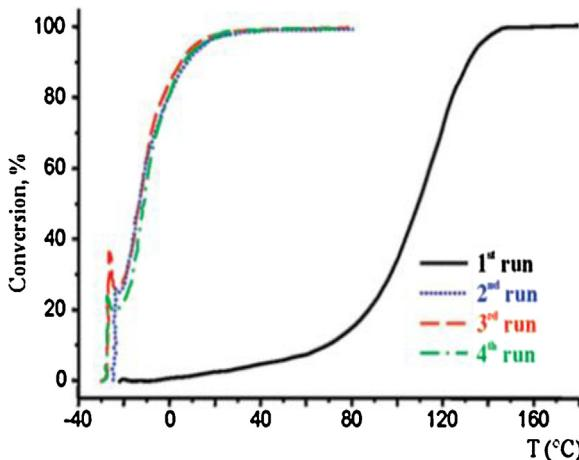
**Fig. 3.** CO oxidation curves for the 1% Au/TiO<sub>2</sub> catalyst (PVA-protected) by the gas mixture (composition, vol%: CO-1, O<sub>2</sub>-20, N<sub>2</sub>-balance), space velocity 80,000 ml/g<sub>cat</sub>/h. From Ref. [87].
