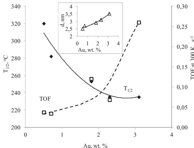
**Fig. 8.** Correlation of turnover frequencies of CO oxidation (TOF) and temperature of 50% conversion CO (T<sub>1/2</sub>) with Au content of the catalysts. Insert shows the correlation of the average size of Au particles with Au content of the catalysts (according to data [89]).
