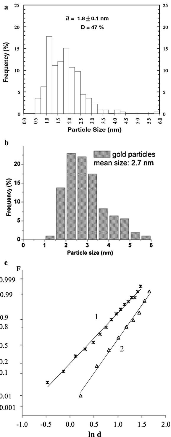
**Fig. 6.** Differential (a and b) and integral (c) gold particle size distribution for Au/CZ-DPU-OE523 (a) and Au/MgFe<sub>2</sub>O<sub>4</sub> (b) catalysts. (c) – Linearization of distributions in the probabilistic logarithmic coordinates; 1 – Au/CZ-DPU-OE523; 2 – Au/MgFe<sub>2</sub>O<sub>4</sub>. Differential distributions from: Ref. [90] (a) and Ref. [88], Supplementary (b).
