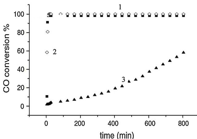
**Fig. 5.** CO oxidation at 25°C using dried 2.6%Au/ZnO catalyst precursors by CO/synthetic air (CO<sub>2</sub>-free) with a molar ratio of 0.5/99.5. Temperature of precipitation of catalysts: 1–60 °C, 2–80 °C, 3–90 °C. Flow rate 20 ml/min, catalyst loading of 50 mg. From Ref. [12].
