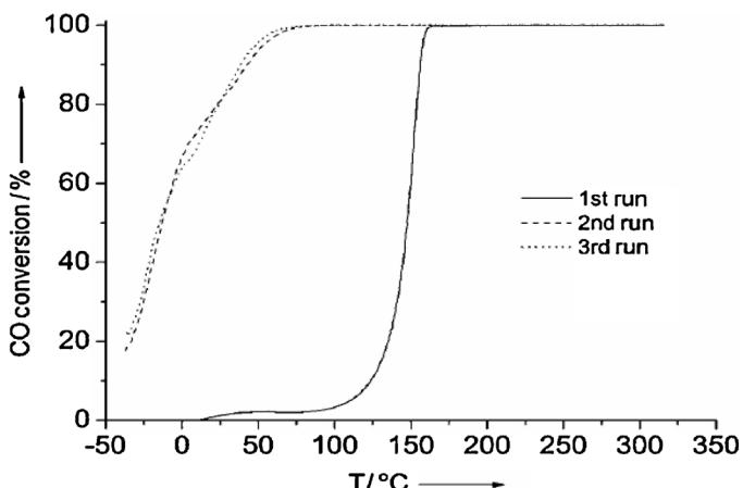
**Fig. 2.** CO oxidation curves for the 1.22% Au/FeO<sub>x</sub> catalyst by the gas mixture (composition, vol%: CO-1, O<sub>2</sub>-20, N<sub>2</sub>-balance), space velocity 80,000 ml/g<sub>cat</sub>/h. From Ref. [83].
