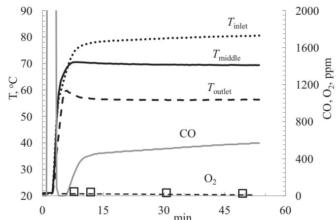
**Fig. 1.** Preferential oxidation of CO over 1% Au/Al<sub>2</sub>O<sub>3</sub> catalyst (a bed height of ~1.6 cm) by the gas mixture (composition, vol%: O<sub>2</sub>–0.9, CO–0.9, H<sub>2</sub>–60, N<sub>2</sub>—balance) at room temperature. Transition into the steady-state CSI. The temperature at the bed: inlet— $T_{\text{inlet}}$ , outlet— $T_{\text{outlet}}$ , and the middle of the bed— $T_{\text{middle}}$ . GHSV 41 Nl/g<sub>cat</sub>/h.
