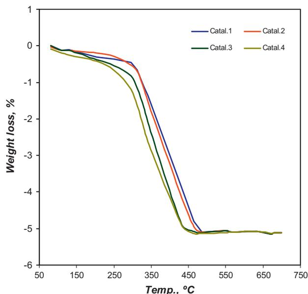
Fig. 1. Thermogravimetric analysis of supported hybrid Cu catalysts **Catal.-1** to **Catal.-4**.
