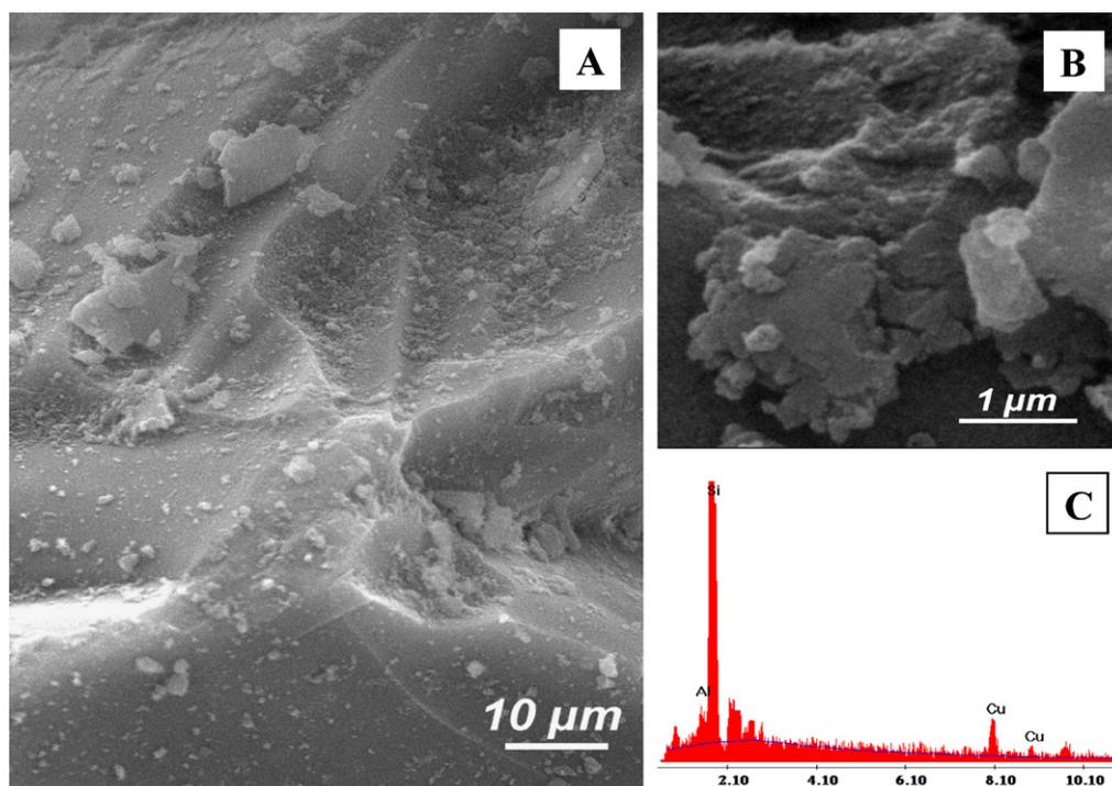
Fig. 2. Scanning electron microscopy images 2 and EDS spectra of **Catal. 2**.
