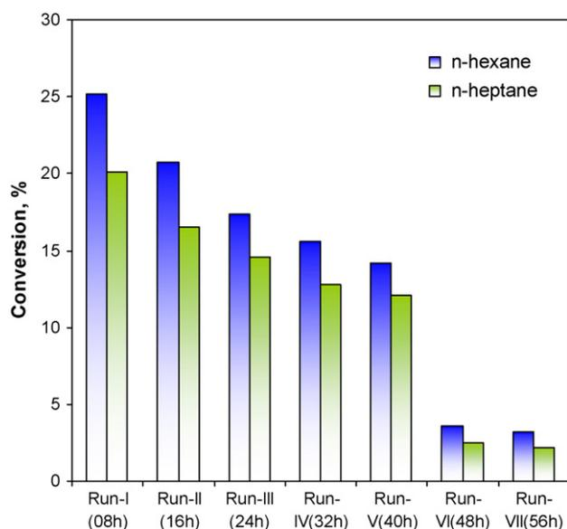
**Fig. 7.** **Catal.-2** recycle tests for *n*-alkanes oxidation under analogous conditions as Table 1.
