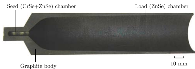
Fig. 1. A crucible used for growth. A vertical section.
