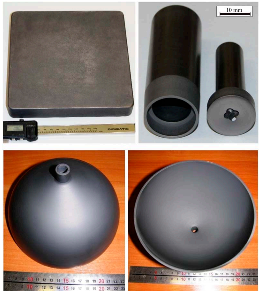
Figure 7. Examples of gas-tight SiC coatings of uniform thickness on the large graphite parts with complicated geometries.
