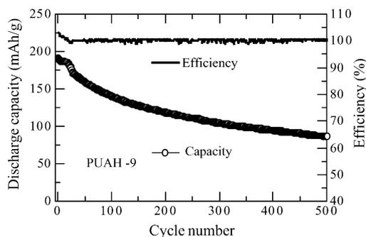
Fig. 12. Cyclic performance of the Li/PUAHI-9/Li<sub>0.33</sub>MnO<sub>2</sub> cell at 60 °C.
