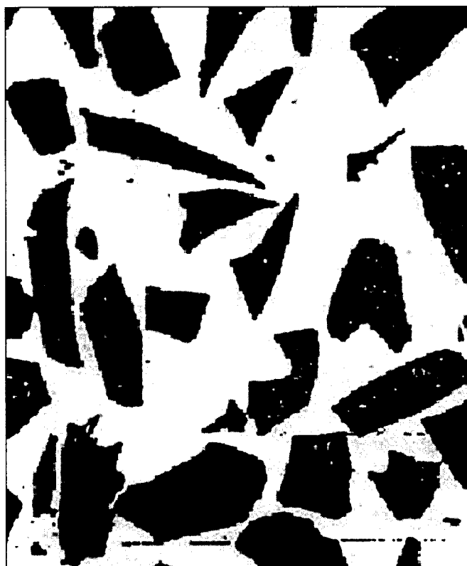
Рис. 10. Микроструктура нового SiC-материала (x70) The microstructure of a novel SiC-based material (x70)
